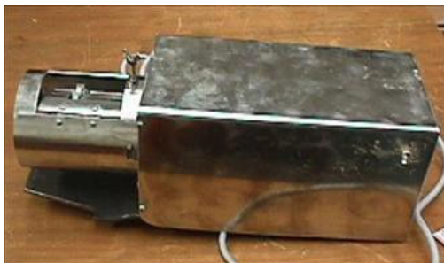
Figure 23—Mechanical stainless steel oyster grinder
