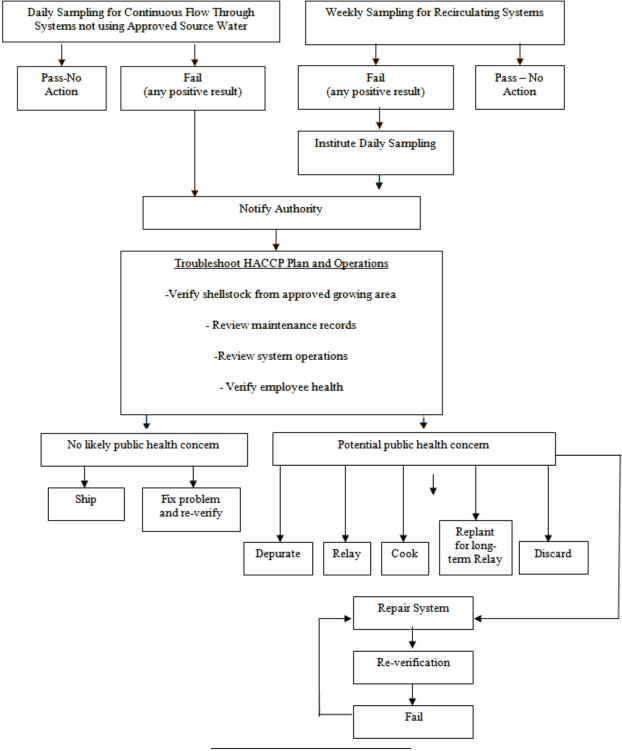
Description: Flow chart showing the protocol for addressing positive coliform results in artificial wet storage water bodies.
