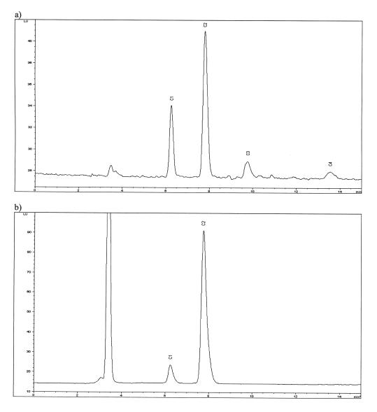
Figure 2. Chromatograms of (a) C toxin mixed working solution (5  $\mu$ L) on a Thermo BetaBasic 8 (4.6 × 250 mm, 5  $\mu$ m). Mobile phase (isocratic): 2 mM tetrabutyl ammonium phosphate, pH 5.8, at 0.8 mL/min. Ox = 5 mM H<sub>5</sub>IO<sub>6</sub>, 100 mM H<sub>3</sub>PO<sub>4</sub>, pH 7.8, 0.4 mL/min; H+ = 0.75 M HNO<sub>3</sub>, 0.4 mL/min. (b) Mussel sample containing 51.4  $\mu$ g STXeq/100 g C toxins, conditions as above.
