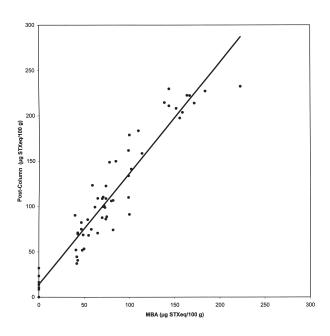
Figure 3. Correlation between results of the MBA method and the new postcolumn method for samples up to 250  $\mu$ g STXeq/100 g; *y* = 1.22*x* + 13.99; r<sup>2</sup> = 0.86.
